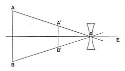
the object AB; thus there is no angular magnification, but rather angular diminution, and the lens is not serving any useful end. If only E could be on the same side of the lens as AB, the angle A'EB' would be greater than the angle AEB, and angular magnification would be attained; but it is impossible to use a lens if the eye is on the same side of it as the object.
